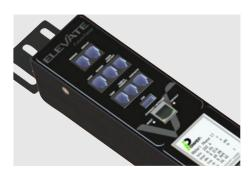
Equipped with ports to connect sensors for temperature, humidity, water detection, or door access sensors, enabling a comprehensive environmental monitoring system.
