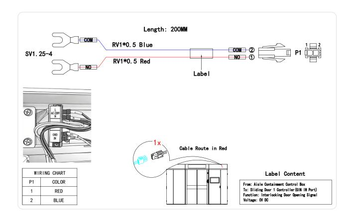
The cable is connected to the Sliding Door 1 Power Controller:
