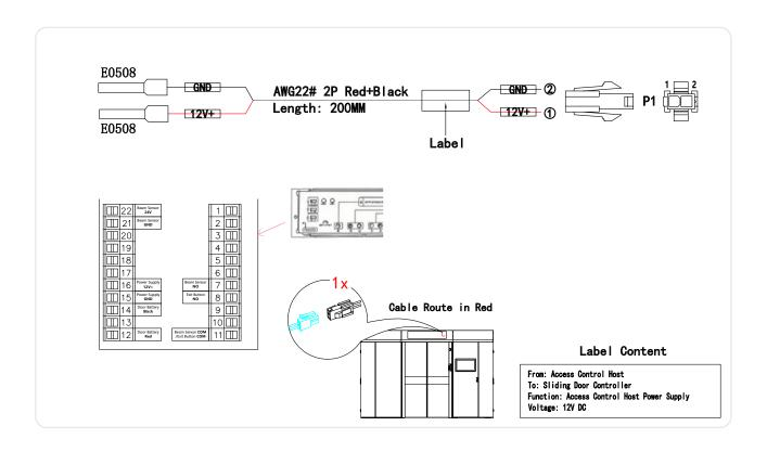
The cable is connected to the Sliding Door Controller (Left side terminal block):
