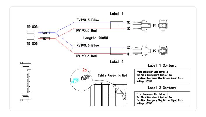
The cable is connected to the Aisle Control Box:
