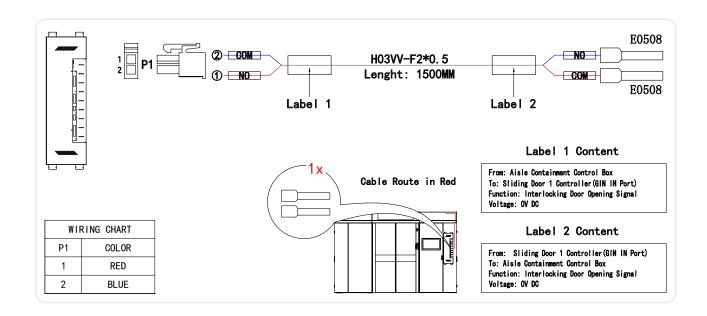
The cable is connected to the Aisle Control Box:
