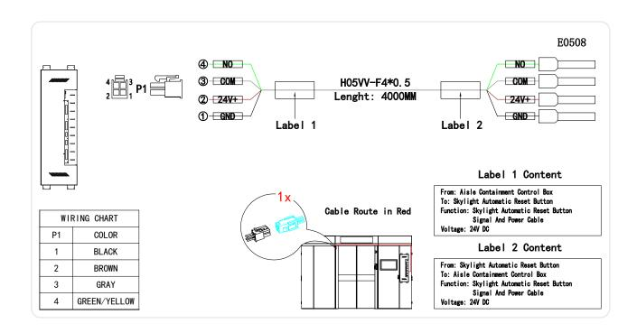
The cable is connected to the Aisle Control Box:
