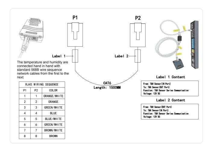
The temperature and humidity are connected hand in hand with standard 568B wire sequence network cables from the first to the next.
