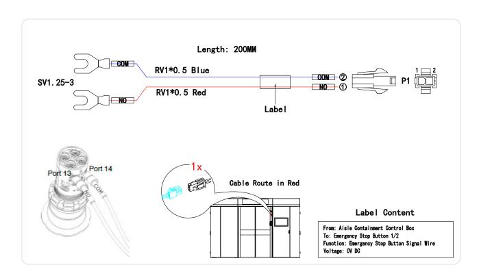
The E-stop Button is installed on the sliding door panel:
