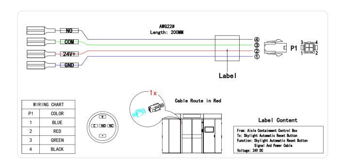
Reset Button terminal wiring configuration:
