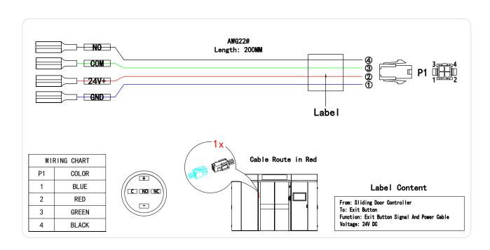
Exit Button terminal wiring configuration:
