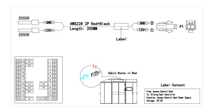
The cable is connected to the Sliding Door Controller (Left side terminal block):
