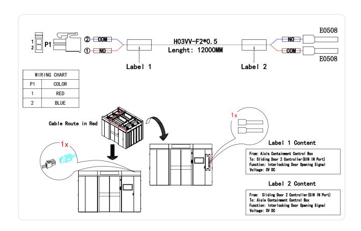
The cable is connected to the Aisle Control Box:
