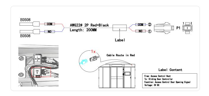
The cable is connected to the Sliding Door Power Controller:
