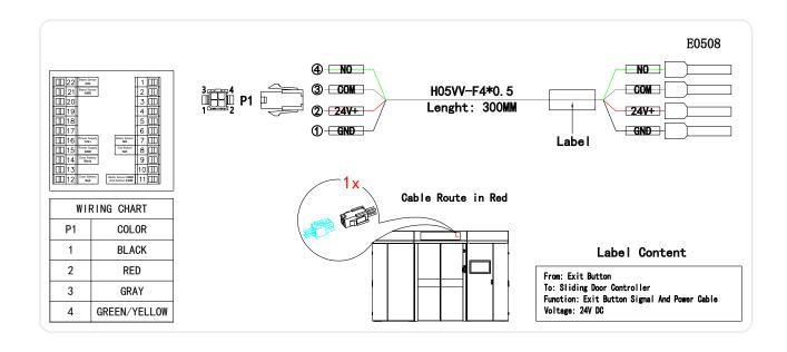
The cable is connected to the Sliding Door Controller (left side terminal block):
