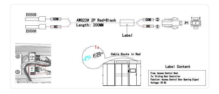
The cable is connected to the Sliding Door Power Controller:
