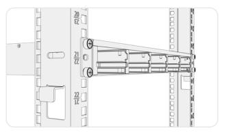
1.5: Tighten all screws ensuring the panel is level and within the designated U space.
