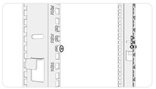
1.3: Mount the panel onto the bottom screw allowing the panel to rest on them.
