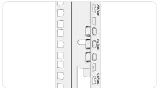
1.2: Install the bottom cage screw each side.
