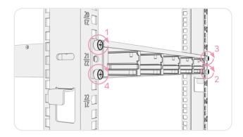
1.6: Install the front management panel using the central cage nut point.
